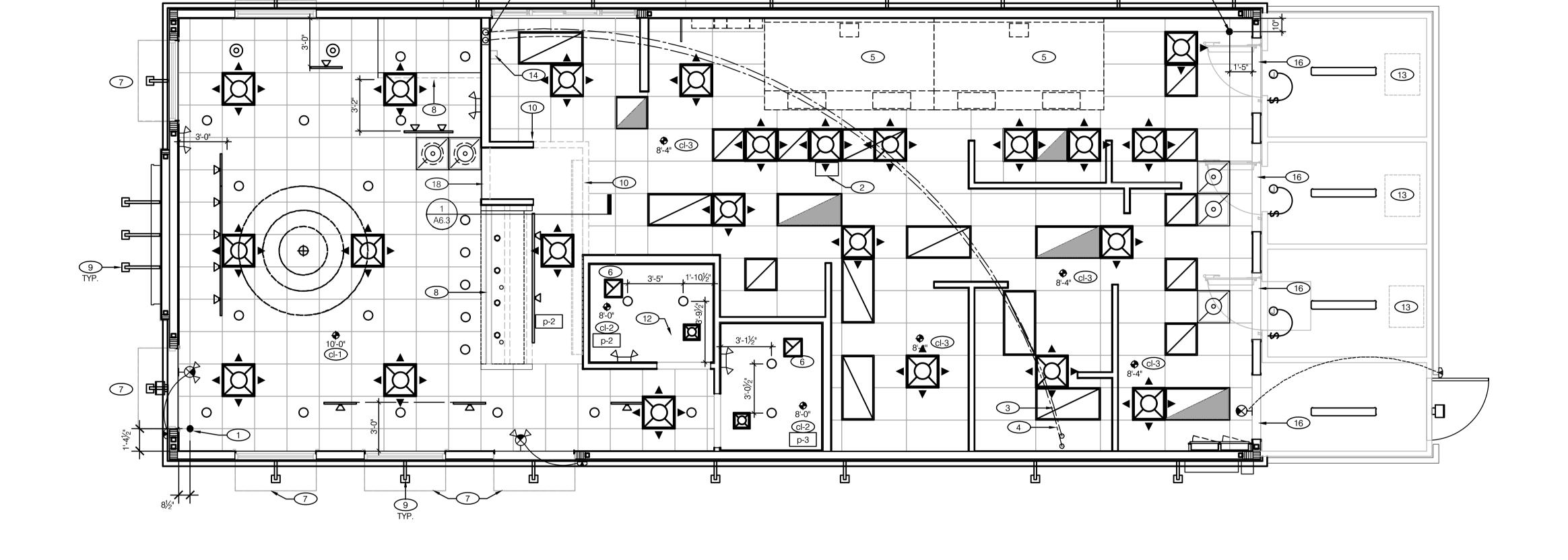
EXTERIOR WALL FIXTURE LED LIGHT **FIXTURE** SPEAKER LED LIGHT 12" EXHAUST FAN **FIXTURE** DOWNLIGHT @ WALK-IN HVAC RETURN GRILLE (BY WALK-IN MFR.) PENDANT FIXTURE HVAC SUPPLY DIFFUSER
