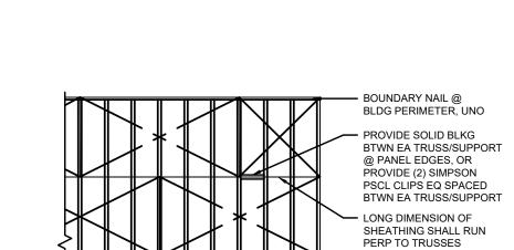
Roof Nailing Plan
