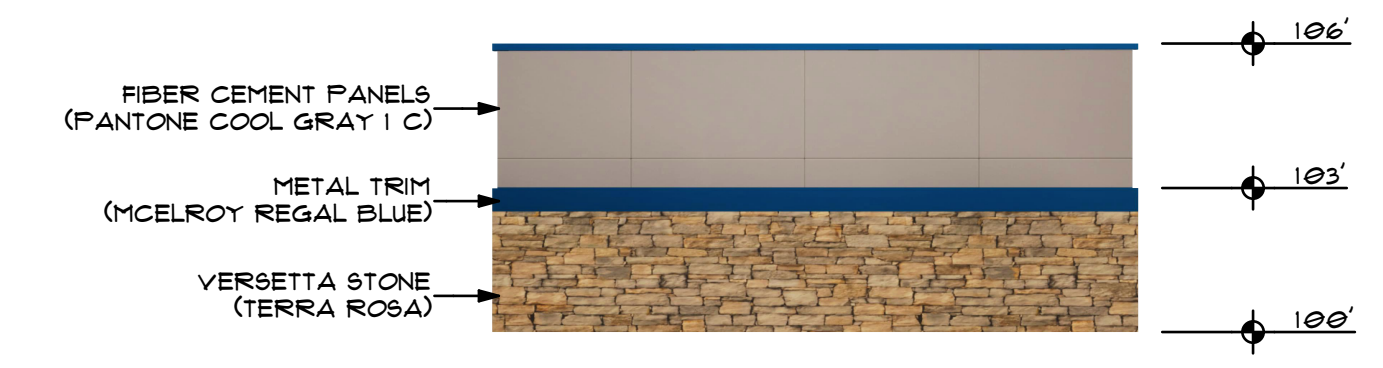
E NORTH - DUMPSTER ENCL. SCALE: 1/4" = 1'-0"
