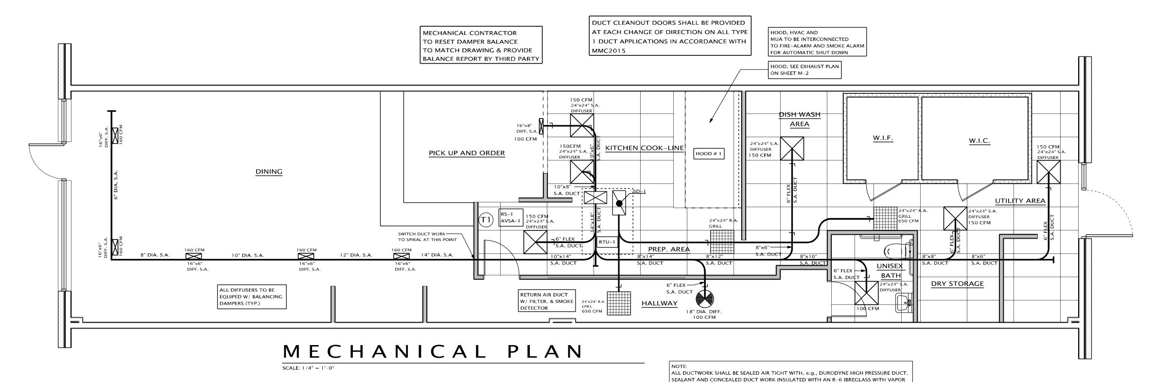
LEGEND EF EXHAUST FAN S.A. SUPPLY AIR RTU ROOFTOP UNIT RETURN AIR AVSA AUDIO VISUAL SMOKE ALARM SUPPLY FAN REMOTE TEMP. SENSOR MUA MAKE UP AIR UNIT | R.S. THERMOSTAT-NUMBER
