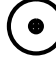
PENDANT HUNG LIGHT FIXTURE. CENTER ON COUNTER OR AS SHOWN. MOUNT WITH BOTTOM OF FIXTURE AT 7'-2" AFF. COORD. W/ MANUFACTURER FOR REQUIRED CORD LENGTH.
