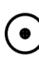
PENDANT HUNG LIGHT FIXTURE. CENTER ON COUNTER OR AS SHOWN. MOUNT WITH BOTTOM OF FIXTURE AT 7'-2" AFF. COORD. W/ JACKSON LIGHTING FOR REQUIRED CORD LENGTH.
