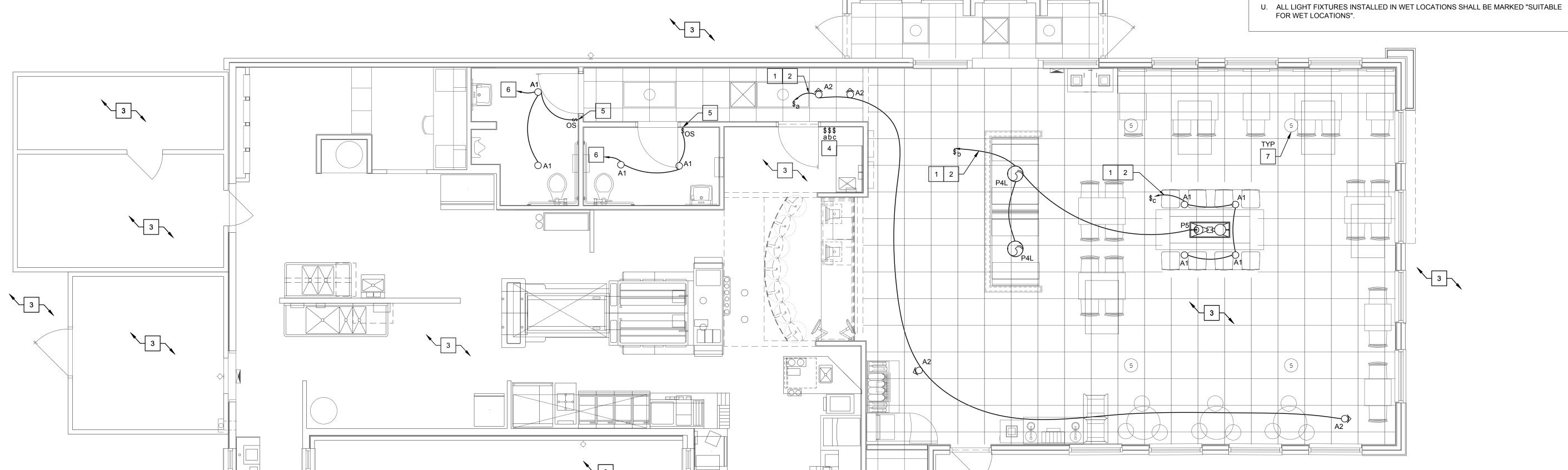
. WIRE ALL NIGHT LIGHT ('NL') AND EMERGENCY FIXTURES AHEAD OF ANY SWITCHING ON CIRCUIT INDICATED.
