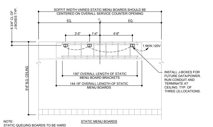
WIRED. G.C. TO PROVIDE J-BOX ABOVE CEILING CENTERED BETWEEN BOARDS.
