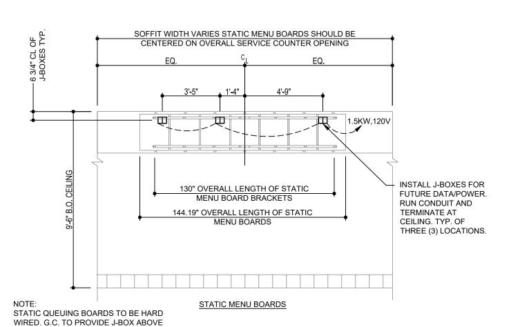
CEILING CENTERED BETWEEN BOARDS. MAIN MENUBOARD ROUGH-IN ELEVATION
