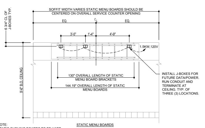
STATIC QUEUING BOARDS TO BE HARD WIRED. G.C. TO PROVIDE J-BOX ABOVE CEILING CENTERED BETWEEN BOARDS.
