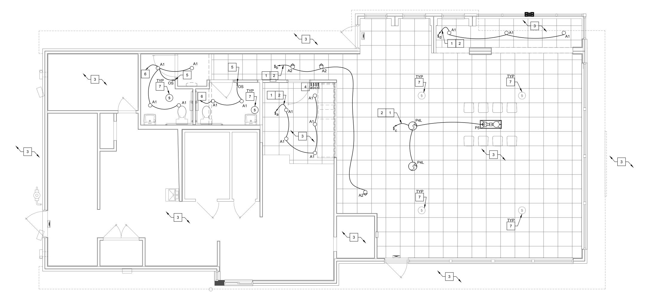
. WIRE ALL NIGHT LIGHT ('NL') AND EMERGENCY FIXTURES AHEAD OF ANY SWITCHING ON CIRCUIT INDICATED.
