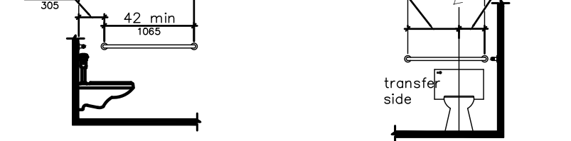
Figure 604.5.1 Side Wall Grab Bar at Water Closets Figure 604.5.2 Rear Wall Grab Bar at Water Closets
