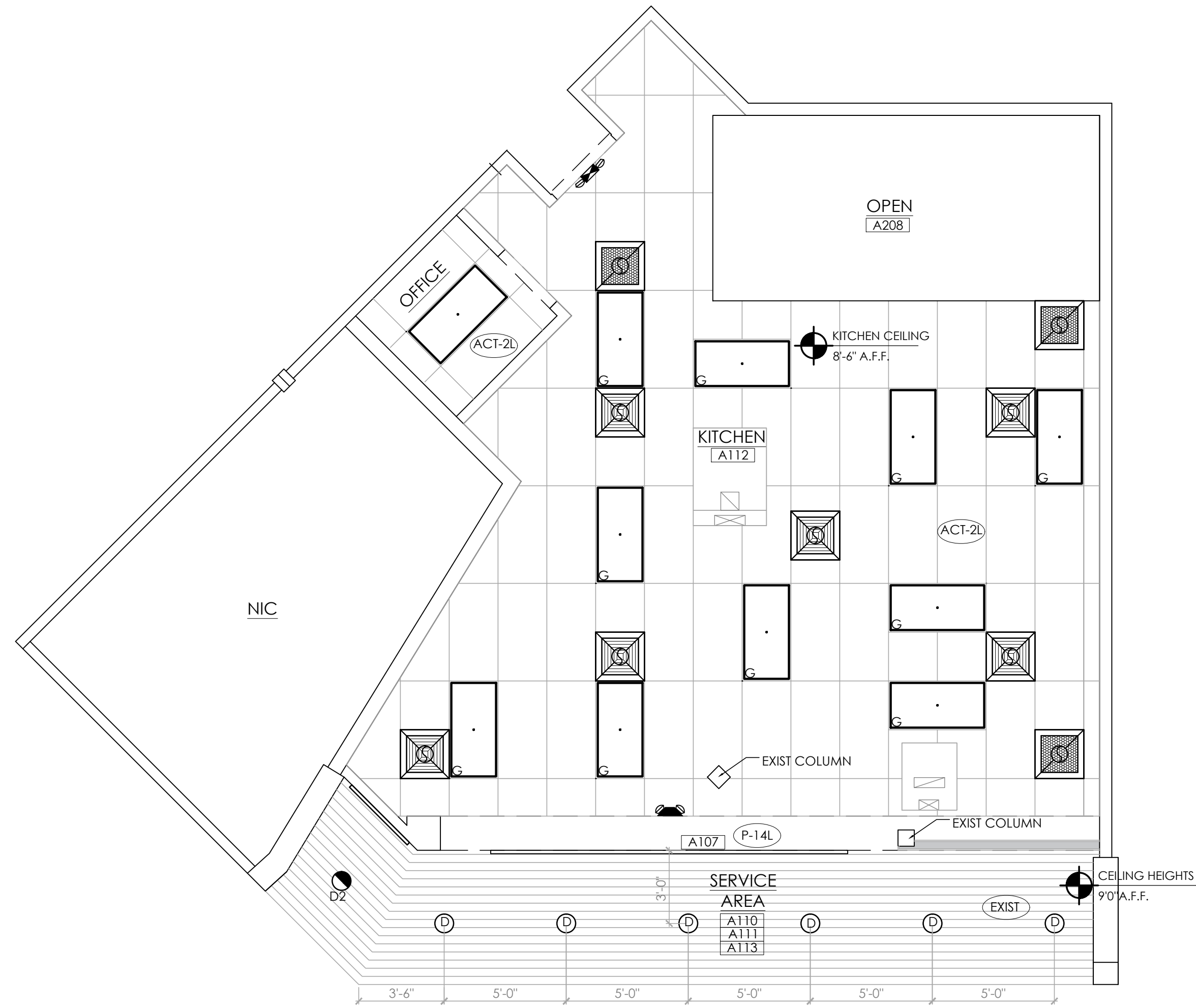
3 REFLECTED CEILING PLAN SCALE: 1/4" = 1'-0"
