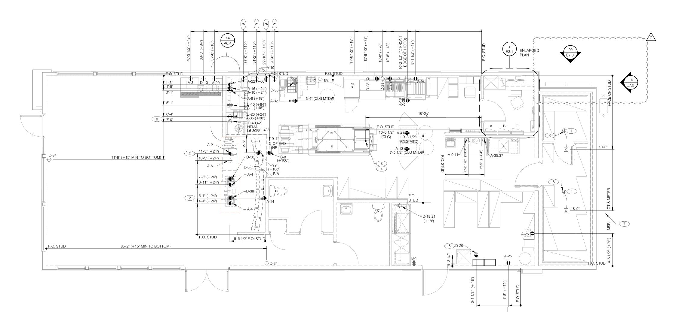
NOTE: IN LIEU OF GFCI OUTLETS YOU CAN USE GFCI CIRCUIT BREAKERS TO SAVE COSTS.
