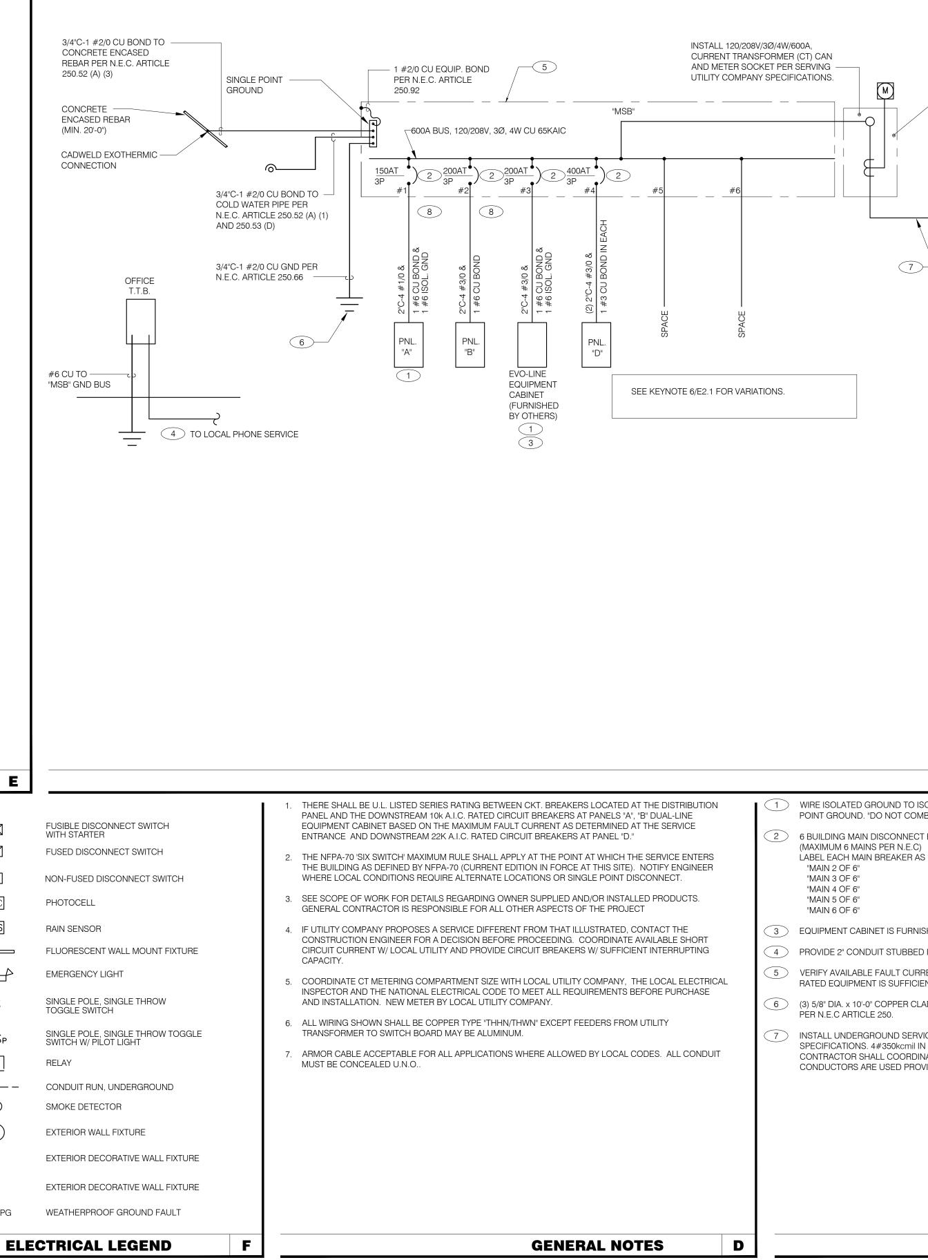
ENGINEER TO CONFIRM WITH LOCAL UTILITY IF CURRENT TRANSFORMERS CAN BE MOUNTED IN UTILITY TRANSFORMER ENCLOSURE AND IF THE METER CAN BE MOUNTED TO THE UTILITY TRANSFORMER ENCLOSURE. IF ACCEPTABLE WITH THE UTILITY, MOUNT CURRENT TRANSFORMER AND METERS AS INDICATED ABOVE IN LIEU OF PROVIDING SEPERATE CT CABINET.
