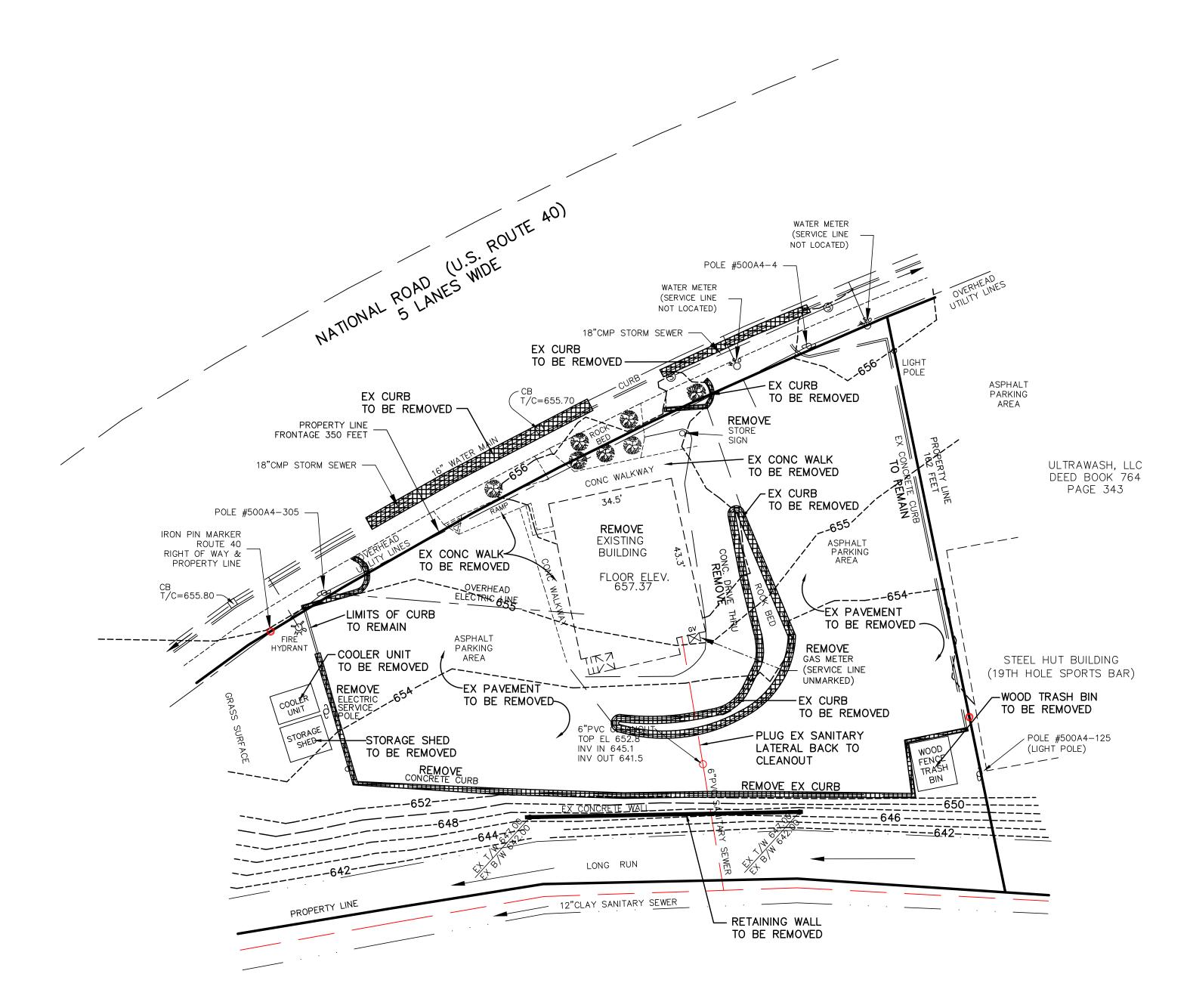
ALL VISIBLE UTILITY LINES AND ASSOCIATED FACILITIES WERE LOCATED BY THE SURVEYOR AS INDICATED ON THIS MAP. THE SURVEYOR IS NOT RESPONSIBLE FOR THE LOCATION OF UNMARKED SUBSURFACE FACILITIES. THE CONTRACTOR MUST CALL MISS UTILITY OF WEST VIRGINIA AT 800-245-4848 (OR DIAL 811) FOR LINE MARKINGS PRIOR TO ANY EXCAVATIONS.
