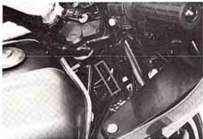
The frame serial number is stamped on the right side of the steering head.
