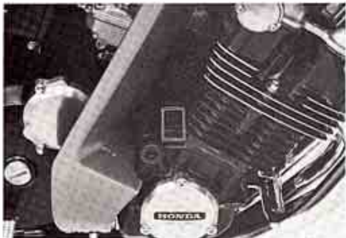
The engine serial number is stamped on the top of the crankcase.
