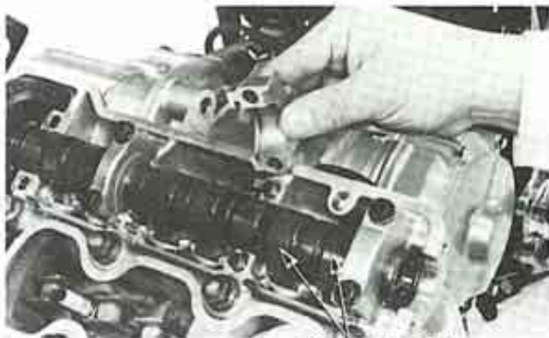
NO. 1 CAM LOBES ALSO, NO. 1 EX. CAM LOBES TOWARD SPARK PLUG.
