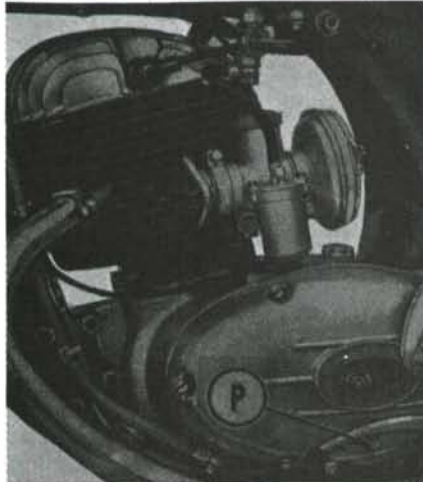
Fig. A3-5—Gear box oil level should be maintained at level of plug hole (P) on 250cc models.
