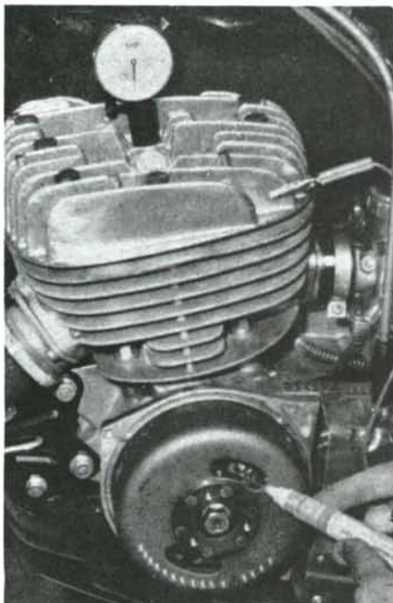
Fig. S12-4—Checking point opening with a dial gage and static timing light. Gage shown is available from Central Tool Co.
