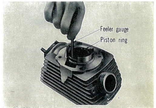
Fig. 6-4-2 Measuring end gap
