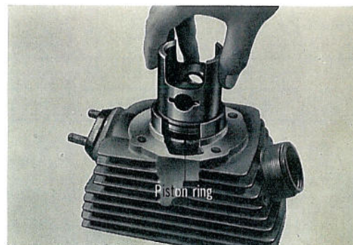
Fig. 6-4-1 Inserting piston ring into cylinder
