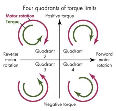
When running OLV, motors can produce 200% of their rated torque at 0.3 Hz. The higher starting torque at lower speeds opens the door for a variety of applications. This control method also allows for four-quadrant torque limits.
