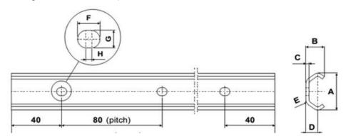
Recommended fastener is a button head cap screw
