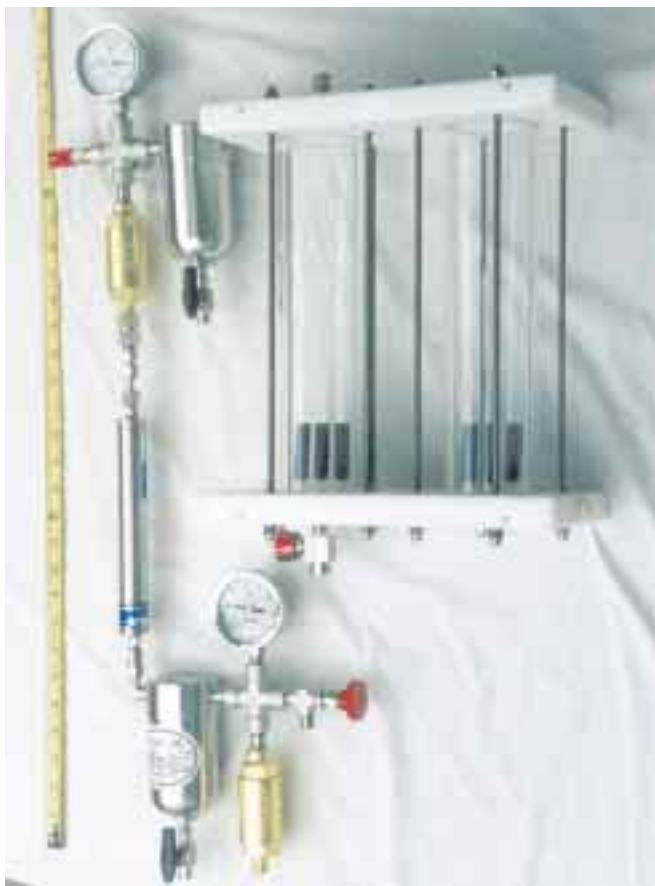
Above: The Double-Bubbler™ and purifier system.
