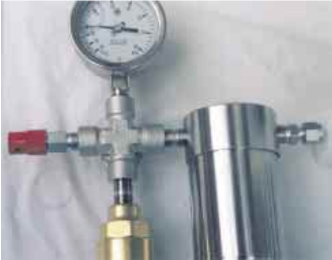
Above: The relief check valve, pressure/vacuum gauge, and tops of a flash-back arrestor and coalescer.
