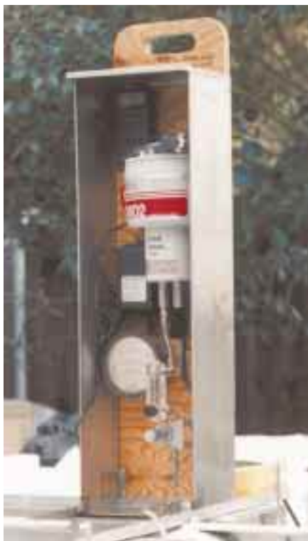
Left: The Panametrics XMO2 oxygen analyzer measures the amount of O 2 contaminant in the hydrogen.
