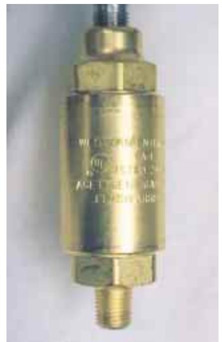
Right: A flash-back arrestor.
